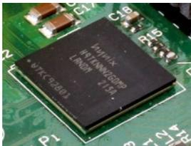
Package-on-package (PoP) is an electronic component-stacked package type consisting of vertically stacked ball grid arrays most
