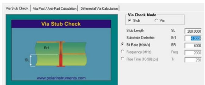
Figure 3: Via length of 200 mils requires attention at 4 Gbit/s data rate. (Find the math behind this in “Signal and Power Integrity Simplified” by Dr. Eric Bogatin)
