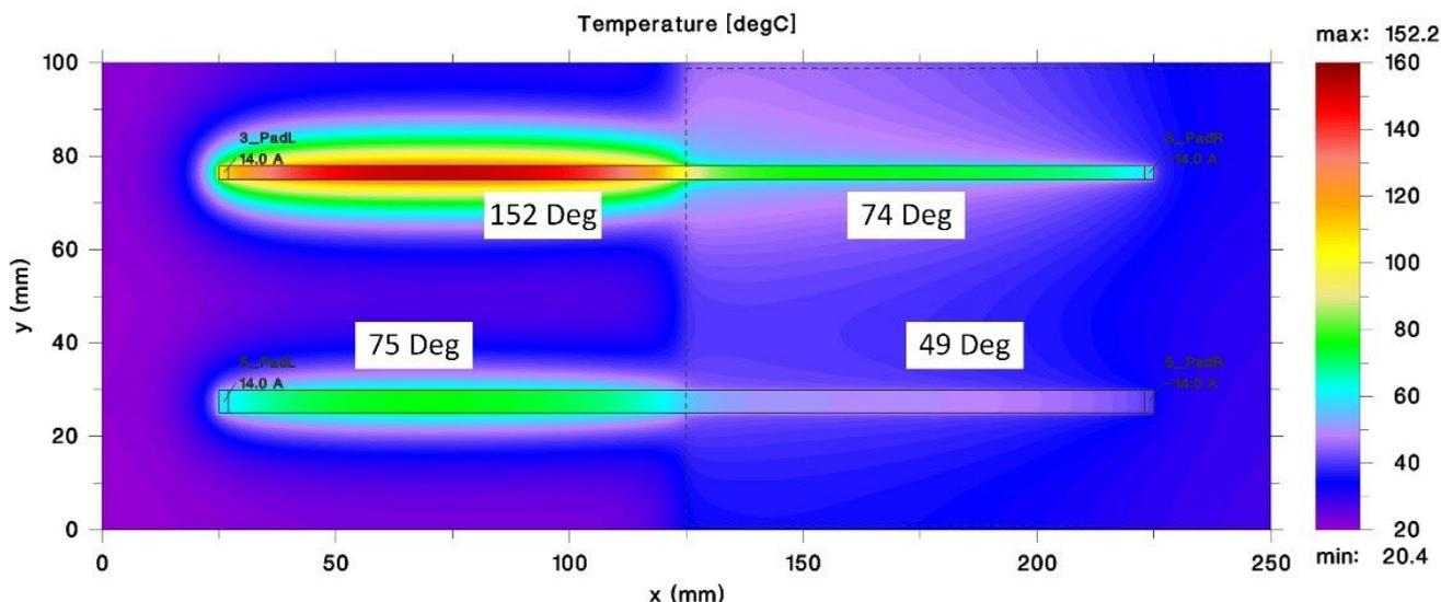
Figure 1: Planar impact on trace temperatures.
