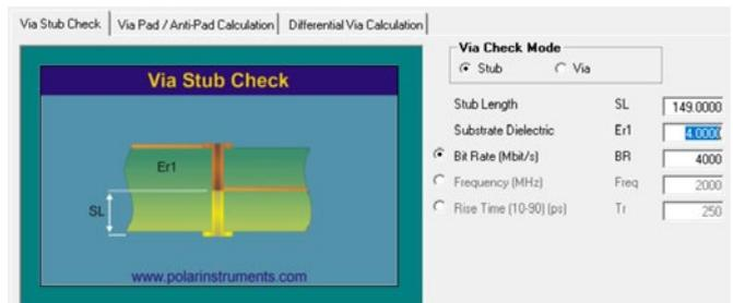
Figure 2: Via length of 149 mils causes some concern at 4 Gbit/s data rate.
