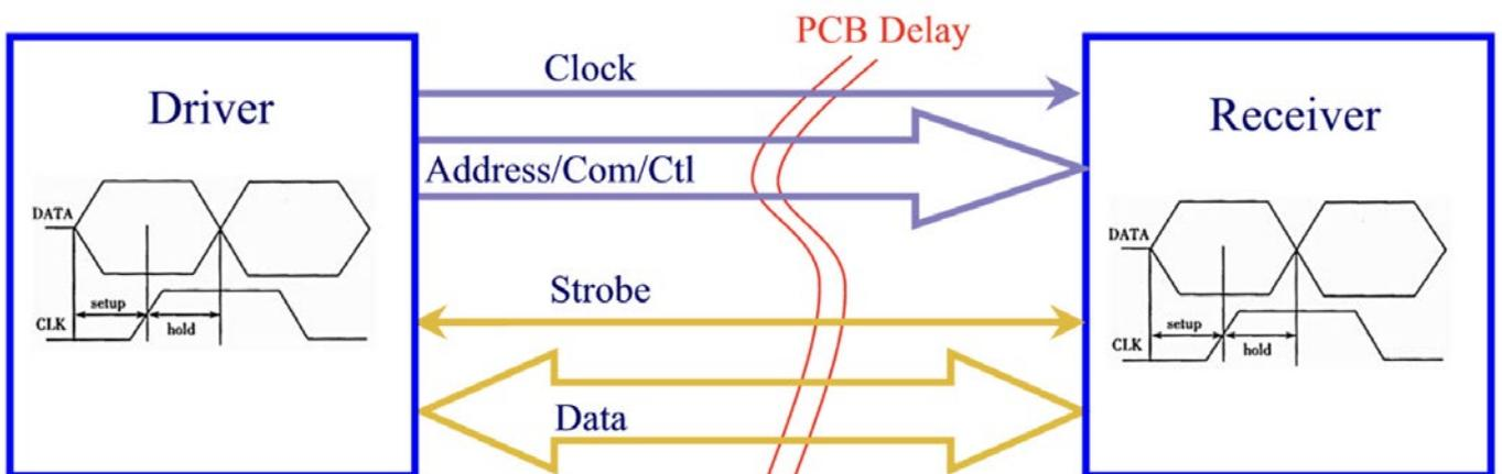
Figure 2: Source synchronous timing relationship across substrate.
