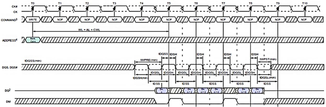
Figure 1: DDR3 synchronous timing. (Source: JEDEC Std 79-F3)
