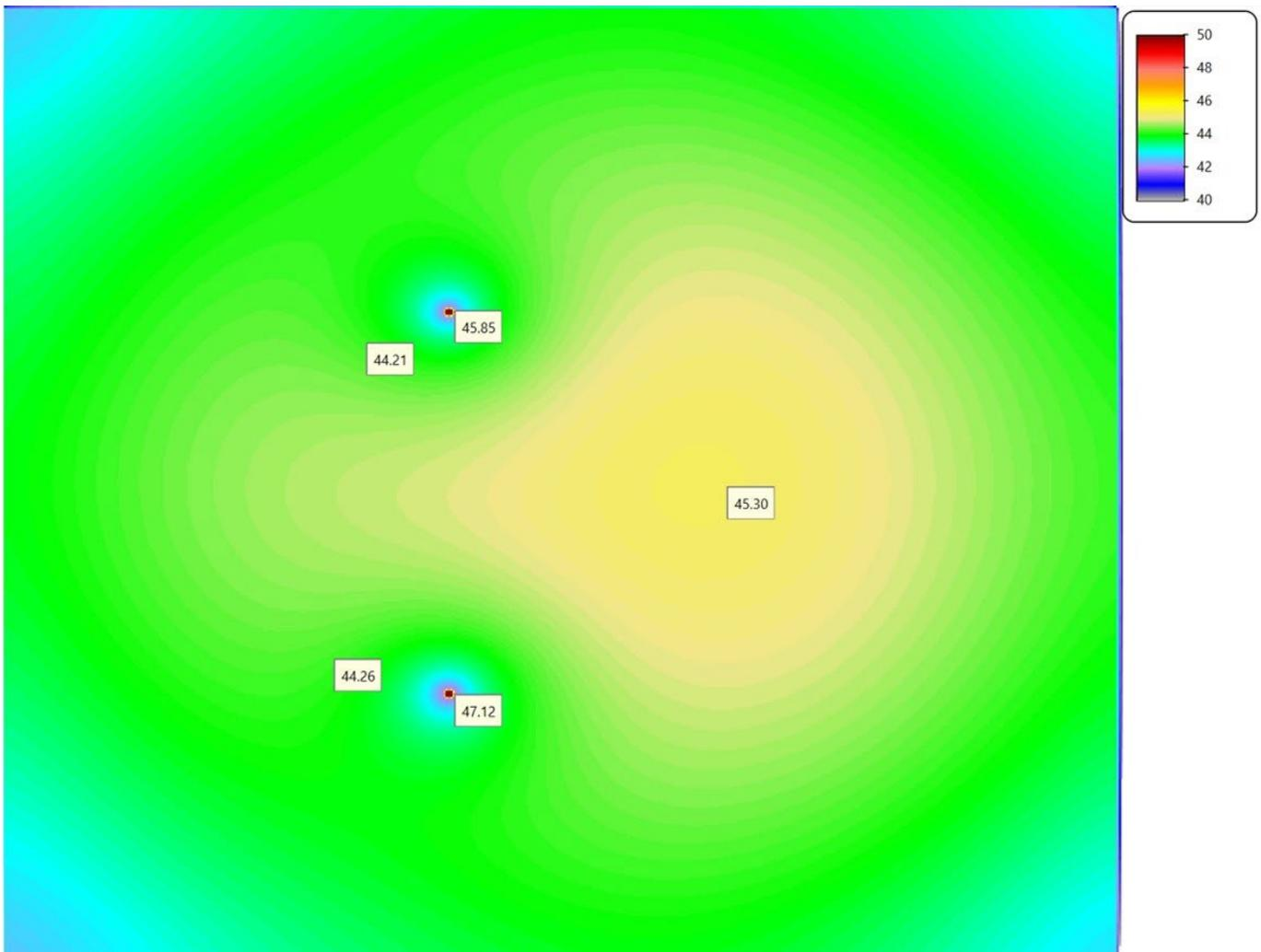
Figure 4: Thermal profile of top pad with two thermal vias.
