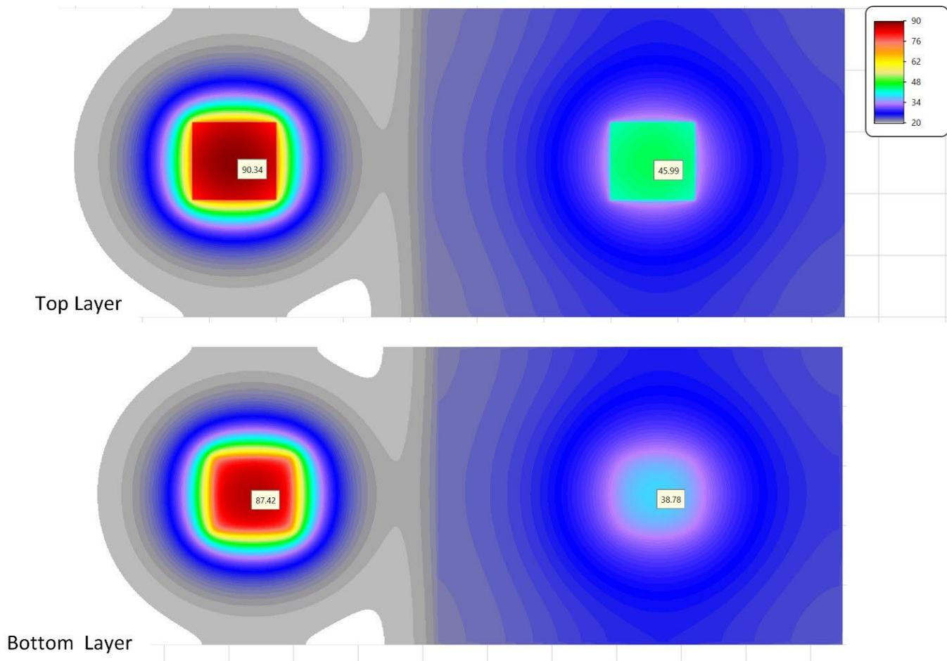
Figure 3: Heated pads, top and bottom layers.
