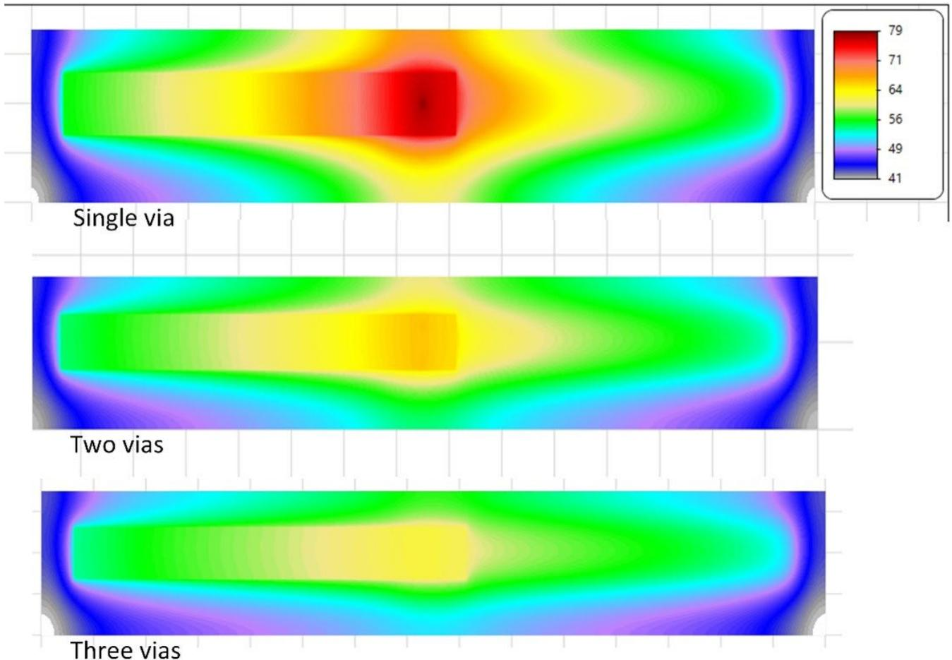
Figure 2: Adding vias lowers temperature to a point.
