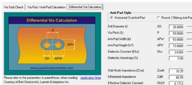
Figure 4: Differential via property calculation, Polar Si9000e. (Courtesy: Bert Simonovich Lamsim Enterprises)
