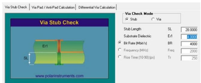
Figure 1: Via length of 28 mils causes no concern at 4 Gbit/s data rate.
